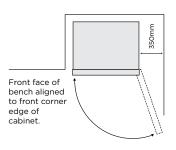
If you have a cupboard above the refrigerator with a rear gap of less than 100mm (Y), recommended minimum clearance at the top of the refrigerator increases from 30mm to 70mm (X).
