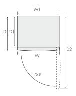
\*For those top mount and bottom mount models with telescopic extension slide-out bins or crispers being placed in location with the door opening against the wall, clearance requirement increases from 350mm to 550mm.
