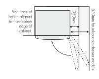
When positioned in a corner area, spacing of at least 350mm on the fridge side will allow the doors to open enough to enable the removal of the crisper bins and shelves. This required clearance inceases to 550mm for those models with telescopic extension slide-out bins.
