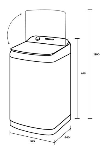
\*Add 25mm for the hose protrusion at the back
