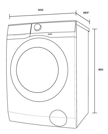
\*Add 20mm for the hose protrusion at the back
